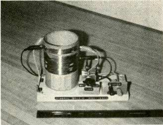
Robert S. Davey's version of the "salt box" crystal set described in Popular Mechanics for January 1977. Clip leads make it easy to experiment with coil taps.
