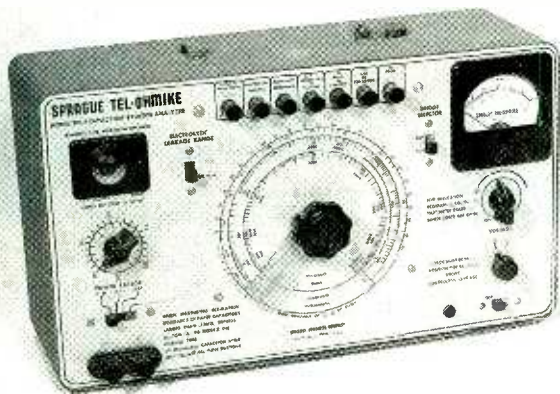
The Sprague TO-4 as received. Its physical condition was good, except for the pushed-in glass window on the meter at the upper right.
