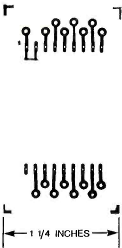
Fig. 3. The LCD display is mounted on its own board. The pattern for that board is shown here full size.
