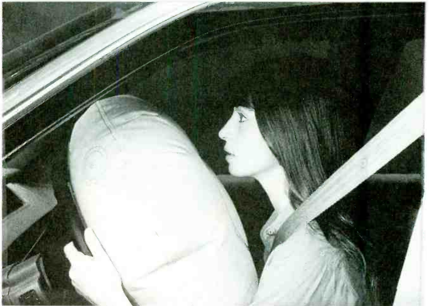
While not a full-sized air bag like those installed in new cars and trucks, the aftermarket SRS-40 from Breed Technologies can provide air bag protection if seat belts are worn.
