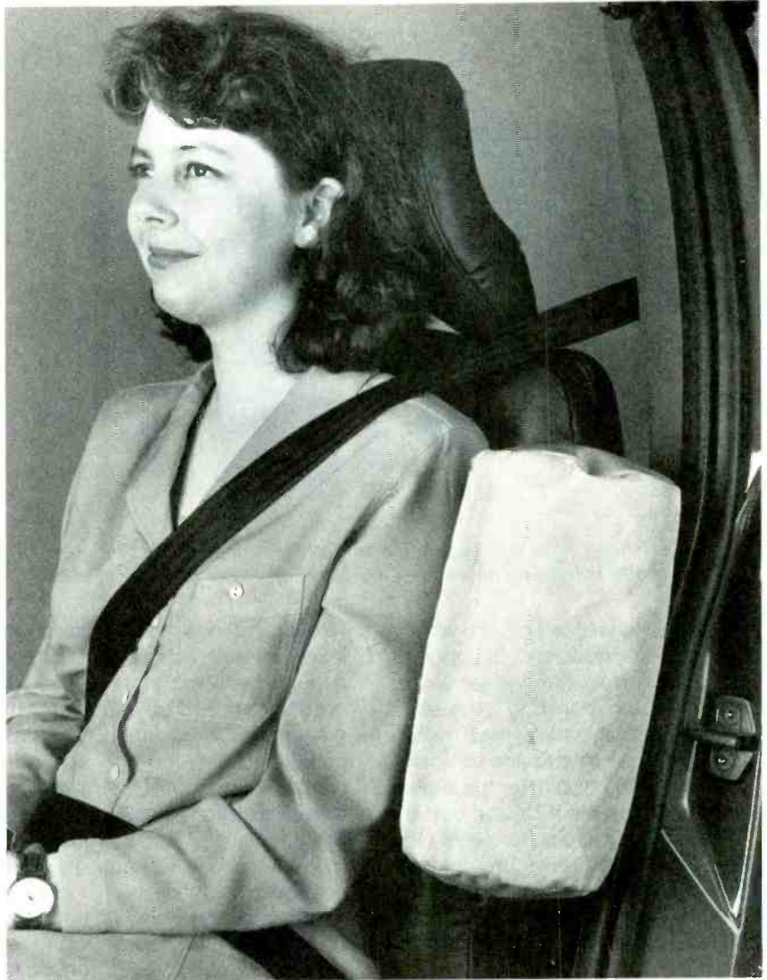
By mounting the bag in the seat rather than the door, the Volvo side-impact air bag is always in the same, optimum position relative to the person in the seat, no matter how the seat is adjusted.
