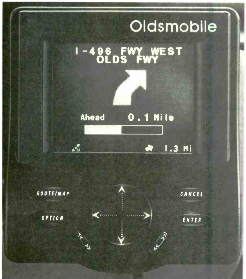
"Turn-by-turn" route guidance provided by simple arrows is augmented by synthesized-voice instructions. The screen also shows the distance to the next required maneuver as well as the direction and distance to the final destination. (Photo courtesy of Oldsmobile.)
