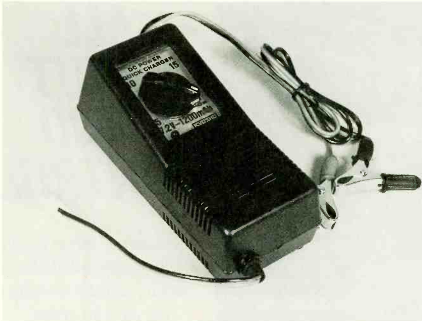
This inexpensive charger, while it can't be plugged into an AC outlet, is all you need (not including a car battery) to charge batteries in the field.
