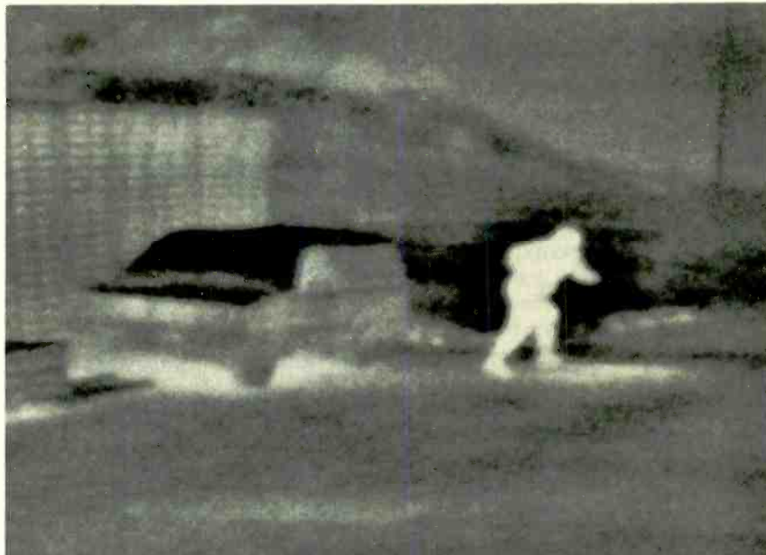
This is what an officer can see on the head-up display or television monitor in a cruiser equipped with the Nightsight system. Notice the extreme visibility of a perpetrator.
