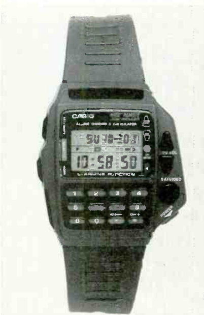
Casio's CMD-40 "Wrist Controller" is a watch, a calculator—and a "learning" universal remote control.
