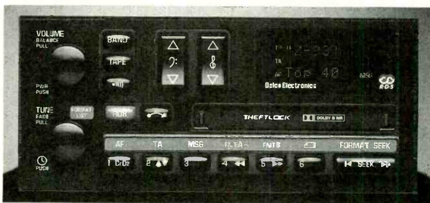
The RBDS receiver/cassette player from Delco receives and decodes the digital RBDS signal, and displays text messages.
