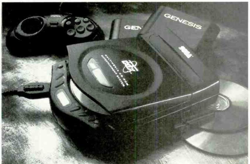
Sega's Genesis CDX can play all cartridge-based Genesis games and all CD-ROM-based Sega CD titles.
