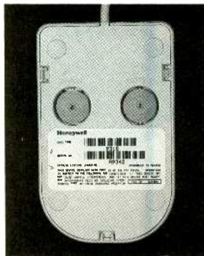
Here's an underside view of the Honeywell mouse. It's lack of a ball mechanism offers some significant advantages over standard devices.
