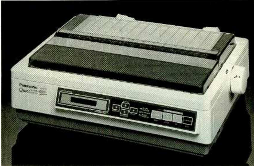
The Panasonic KX-P2124 is a 24-pin LQ impact printer with eight built-in fonts, optional color-printing capability, 360 × 360 DPI graphics resolution, 320 CPS draft speed (about 4 PPM), and two levels of quiet printing. It's under $300 on the street.
