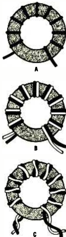
Fig. 1. These toroid cores: are A) single wound; B) bifilar wound (three wires would be trifilar wound); and C) twisted bifilar wound.
