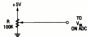
Fig. 3. You should make sure your ADC can produce all the data values from 0 to 255 by using a simple potentiometer connected as shown to simulate a transducer.
