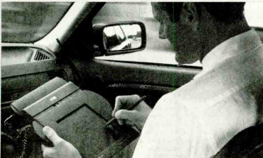
The AT&T EO 440 is a stand-alone mobile office that functions as a cellular phone, portable fax, modem, and notebook computer.
