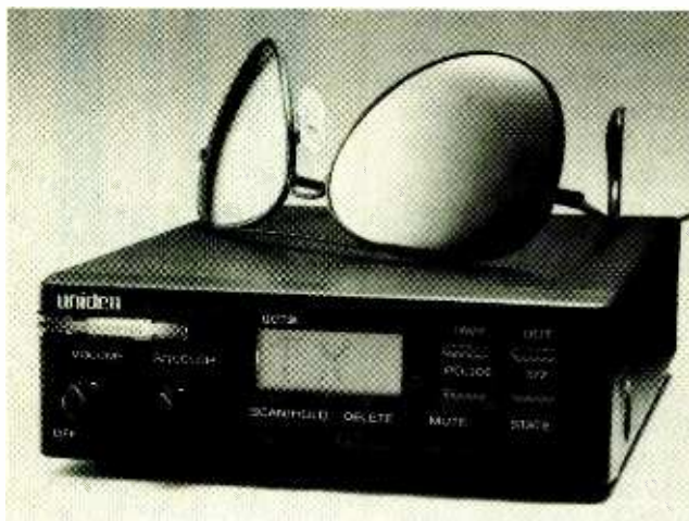
The Bearcat Bear Tracker BCT-2 scanner sounds an alarm when it picks up signals on a highway-patrol frequency.
