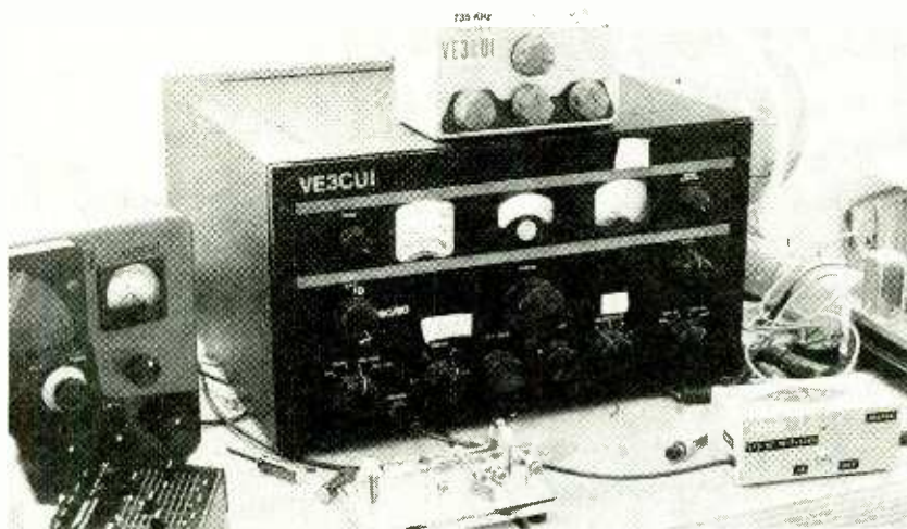
While all the gear in this photo may not be strictly 1950's, most of it is definitely vintage. The centerpiece in this Canadian station is a 1944 RCA AR-88LF receiver. Sitting atop it is a 1950's-era Heathkit Model QF-1 "Q-Multiplier," for improved receiver selectivity. To the left is a Johnson Ranger AM and CW transmitter.
