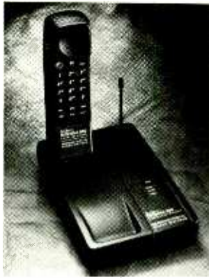
Cobra's Intenna 900 is a 900-MHz cordless phone. Although it operates between 902 and 928 MHz, you won't hear it on your scanner!
