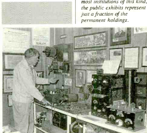
Museum curator Bruce Kelley demonstrates a 250-watt late 1910's or early 20's amateur-radio transmitter, a non-sync rotary spark job. Partly visible on the wall at the upper right is a portrait of Zenith Radio founder R.H.G. Matthews. The brand name was derived from his ham call letters, 9ZN.
