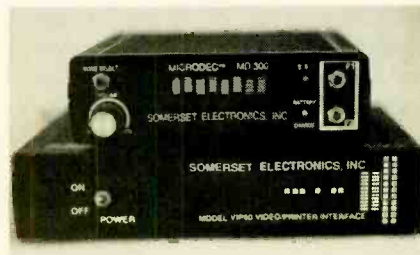
The Microdec decoders let you decode radio transmissions without a computer. They sport an 8-character LED display with intensity controls, a built-in code-practice oscillator, an internal speaker, and pushbutton operation. An optional display adapter, the VIP50 adapter interface (also shown here), offers an expanded display for use with your TV, computer monitor, or VCR.
