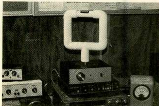
One way to improve receiver reception is to use a loop antenna, such as the square-loop unit from Palomar Engineers.
