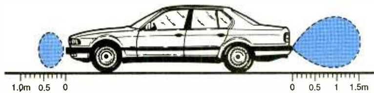
Fig. 3. Detection zones for the PDC system tend to be tight around the front of the vehicle, but less snug toward the rear.
