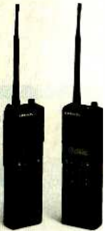
The 2.5-watt, 800-MHz LTR 8565 from E.F. Johnson Company is an example of a trunked handheld.
