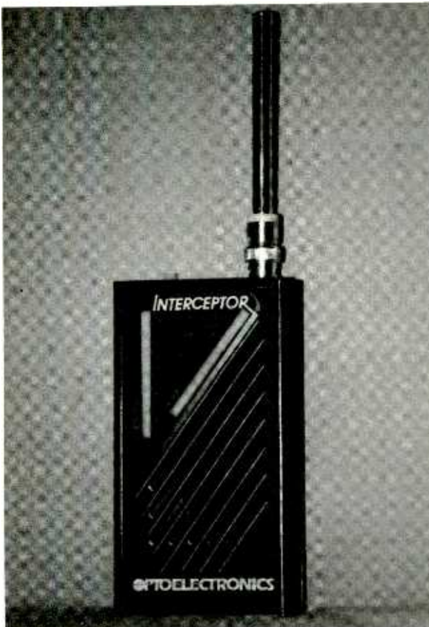
Optoelectronics' R10 FM Interceptor locks in on all close-proximity FM-signal sources, making it ideal for testing communications or locating hidden "bugs."
