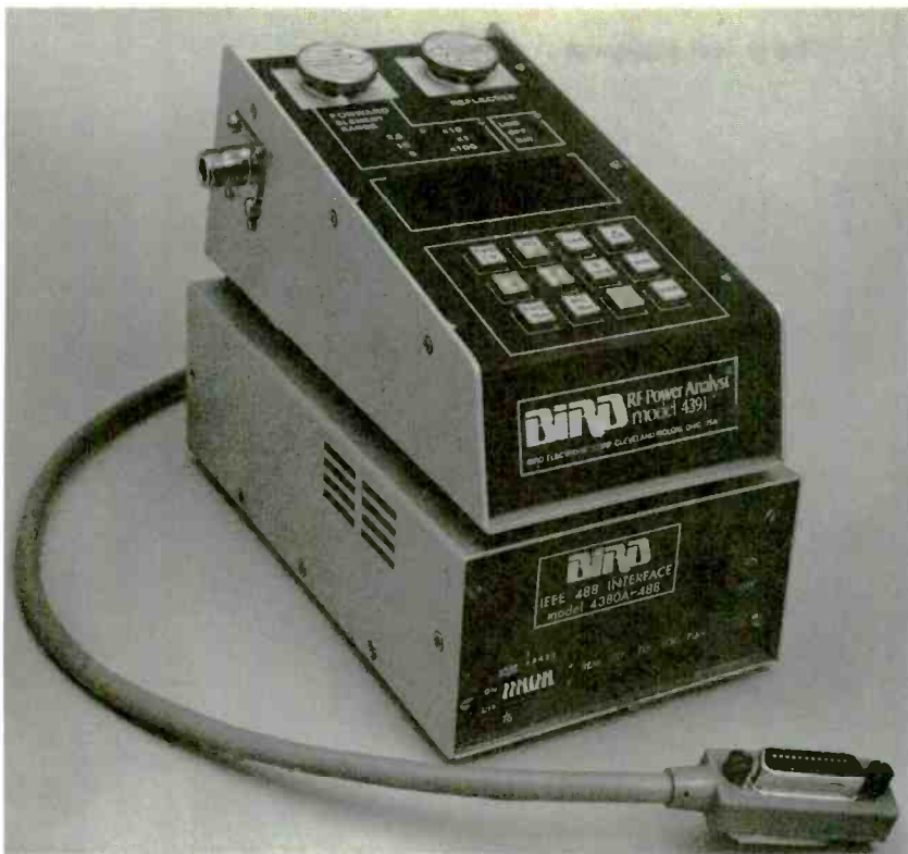
Shown here is the Bird Model 4391 Power Analyst, a high-accuracy and expensive bus-compatible digital-display RF-power and SWR meter. It is best suited for commercial and laboratory installations and those amateurs who insist on professional-quality instrumentation.
