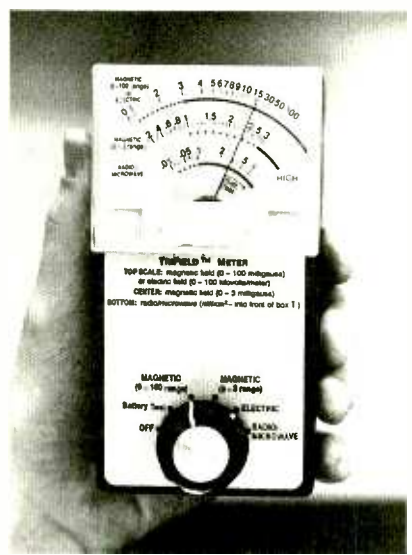
AlphaLab offers its $140 TriField electromagnetic pollution meter that measures both alternating electric and alternating magnetic field strength. It also indicates radiomicrowave power and the full (three-axis) magnitude of field strength.
