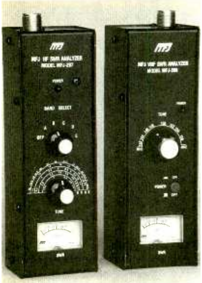
The MFJ-207 HF and MFJ-208 VHF SWR Analyzers physically resemble old-style dip meters, but the analyzers contain a built-in SWR bridge and RF source. When you sweep the band within which the antenna is supposed to be resonant, you get an estimate of the antenna's resonant frequency by observing the dial frequency at which the SWR dip occurs.
