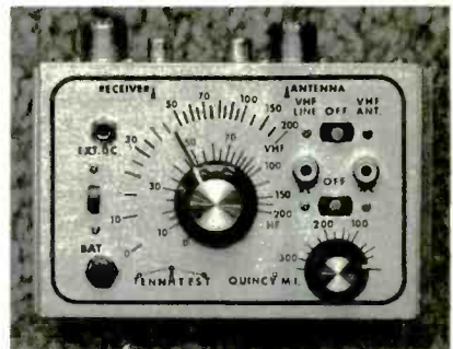
The Tennatest antenna noise bridge offers several useful RF-measurement capabilities, including the determination of resonant frequency of a tuned circuit or antenna, the SWR at resonance, resistive impedance, inductive reactance, and capacitive reactance.
