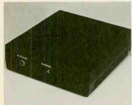
An external antenna plugs into J1 and an 8-ohm speaker or earphones plug into J2.
