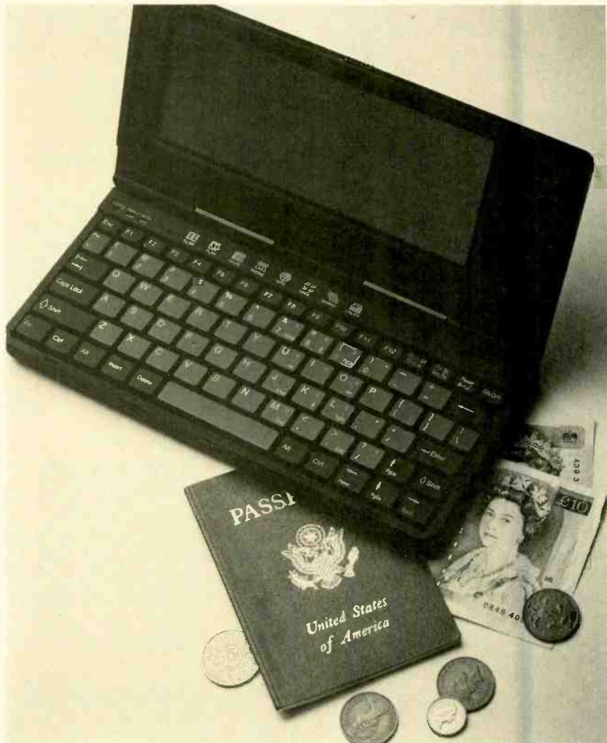
The palmtop ("pocketable") PC is a real PC that runs DOS and has good expandability. Palmtop punch is all the portable PC power needed to send and receive E-mail, modem a memo home, write reports, create spreadsheets, figure expenses, or manage an appointment calendar. This 1.3-lb. ZEOS Pocket PC boasts at least 10 hours on two AA alkaline batteries using power management features that let the computer "doze" or suspend operations to increase battery life.
