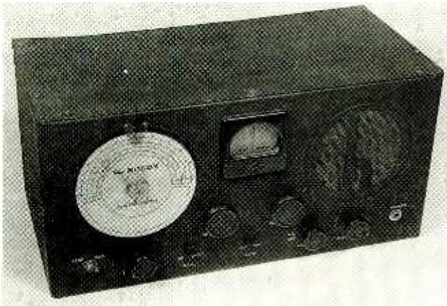
The Sky Buddy with its cover back on and ready for the display shelf. I decided to leave the original dial pointer (which has a broken tip) in place, rather than craft a replacement.
