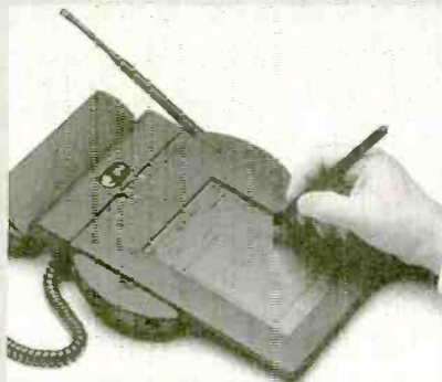
The AT&T Personal Communicator 440 is a pen-based, hand-held device that integrates computing and communications capabilities.
