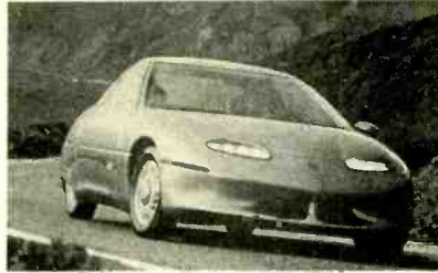
GM's prototype EV, the Impact, has a tear-drop-shaped profile that reduces aerodynamic drag. The Impact's introduction has been delayed until the late 1990's, due to the "high level of uncertainty in the marketplace," according to GM.
