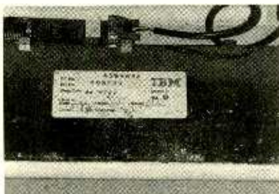
With the bottom removed, all of the dirt trapped within the keyboard comes into view. Shake and brush away the particles.
