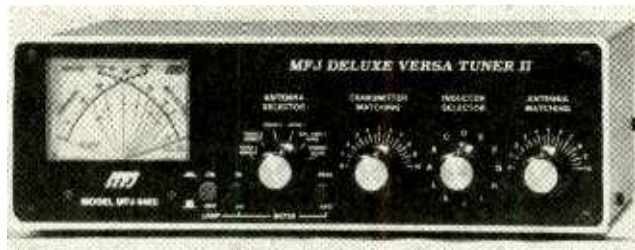
The Deluxe Versa Tuner II, from MFJ Enterprises, Inc., uses a "crossed needles" VSWR meter, which allows you to clearly see the increase in forward power vs. the decrease in reflected power (which represents VSWR).
