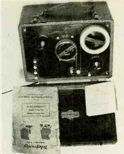
An Instructograph AC-powered code-practice machine. This model had a built-in oscillator. The knobs were used to control volume and speed.
