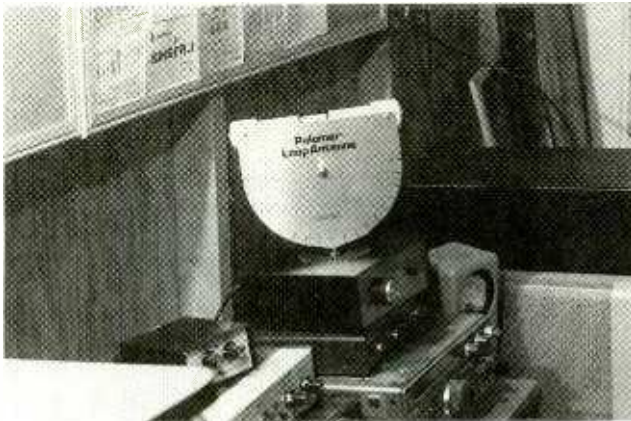
Some hams use loop antennas as receive-only antennas on 75/80-meters in order to weed out QRM from other stations and some man-made noise. Palomar Engineers manufactures a pair of loops; one of which is the loopstick-style unit shown here.
