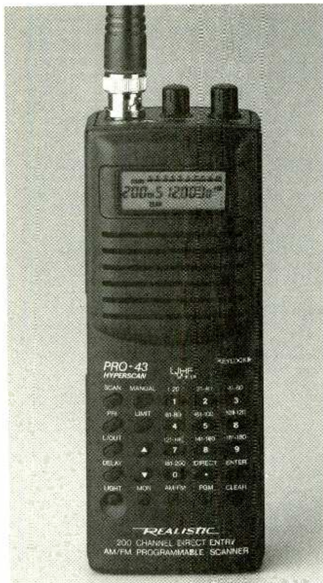
Radio Shack's Realistic PRO-43, with 200 programmable memories, covers the popular military UHF band.
