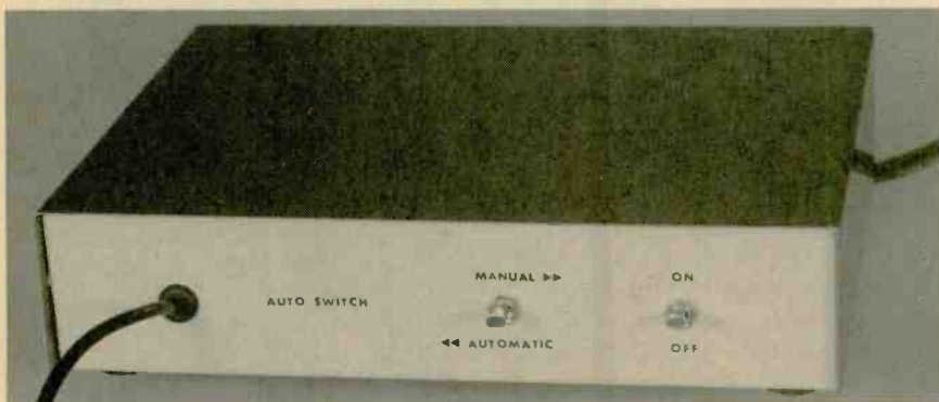
Once the project enclosure has been drilled, labels can be affixed to the front and rear panels to indicate switch functions, and outlet designations.
