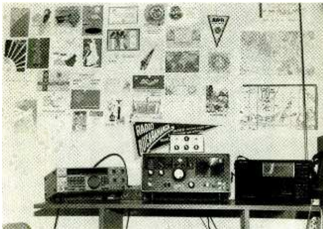
Clifford Nadiger copies shortwave fax transmissions using the setup shown here. His RadFax decoder sits atop an aging Yaseu FRG-7 receiver (center). They are flanked by a Kenwood R-500 at the left and a Radio Shack DX-440 at the right.
