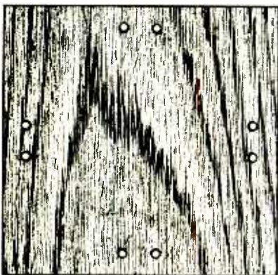
Fig. 1. The 10-Meter version of the Quick And Dirty Quad should be mounted on a TV-antenna rotator and tripod. Four pairs of holes should be drilled in the plywood in this configuration. The spacing and diameter of each pair of holes depends upon the U-bolt chosen to pass through them.
