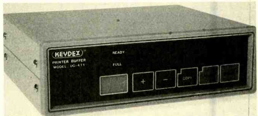
The UG-411 Spooler Buffer from Computer Friends has four status LED's as well as a 2-digit display that indicates the number of copies requested.
