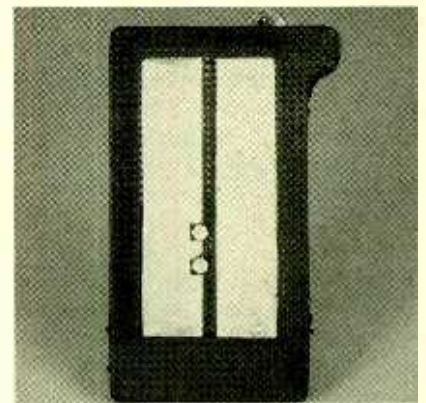
The metal tape strips run almost the full length of the unit. The hardware that holds the stationary clip in place is visible from this perspective.
