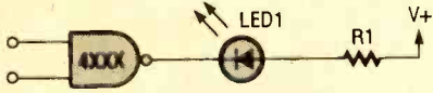
Fig. 6. A CMOS-based gate can sink current much like a TTL gate in order to activate an LED.
