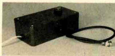
The entire circuit is built on a piece of perfboard, and it all fits inside a small plastic project case. A BNC connector is used to connect the device to an oscilloscope.
