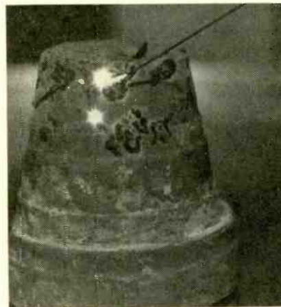
Fig. 2. Two fireballs have spontaneously formed within fissures in the clay pot's surface. Note that the discharge is hot enough to permanently etch black tracks in the clay.
