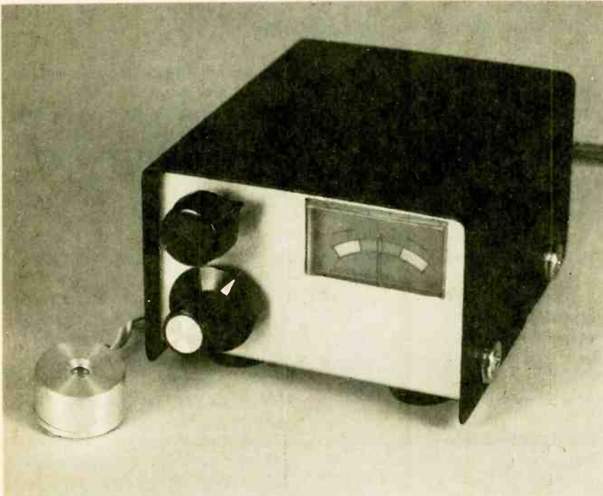
All of the electronics for the Enlarging Light Meter, except for the LDR, were housed in a small enclosure on whose front panel switch S1, potentiometer R14, and meter M1 are mounted. The LDR was housed in a separate enclosure about the size of a bottle cap, and connected to the circuit by wire leads.
