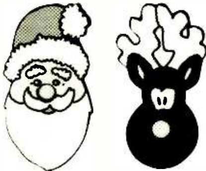
Fig. 2. Shown here are two full-size templates of the faces used by the author. Each has a 3/16-inch hole in the nose, through which the LED will protrude.
