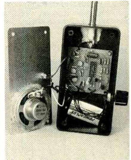
The antenna and speaker for the Countersurveillance Monitor are held in place with silicone cement.
