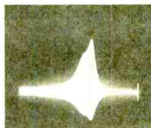
Fig. 6. Shown here is RF response (not rectified) of a 455-kHz IF transformer.
