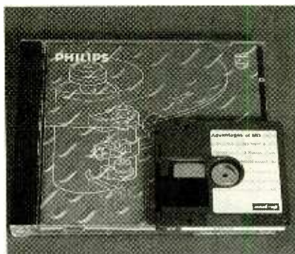
The Mini Disc is only 2.5 inches (2.7 including the caddy). Yet it holds as much music—74 minutes—as does a standard CD.
