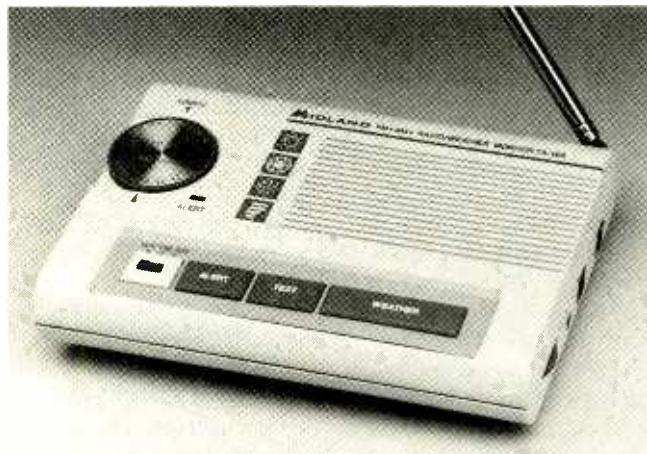
Midland's WeatherMax 74-104 VHF weather monitor offers a couple of bonuses: AM/FM reception and a siren to signal any severe-weather alerts.
