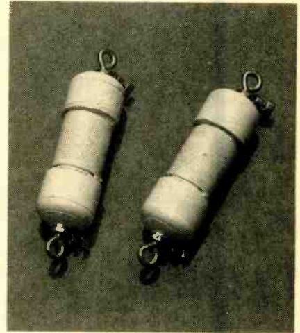
People with space limitations can use shortened dipoles with coils such as these in the two poles.
