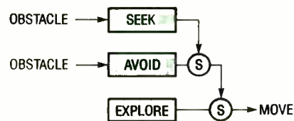
Fig. 3. Our robot will have three basic behaviors that will cause it to explore its world, avoid obstacles, and seek out objects.
