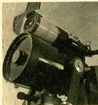
This is an electronically controlled search telescope with top-mounted biosensor assembly. The Faraday tube is shuttered to prevent electromagnetic interference.
