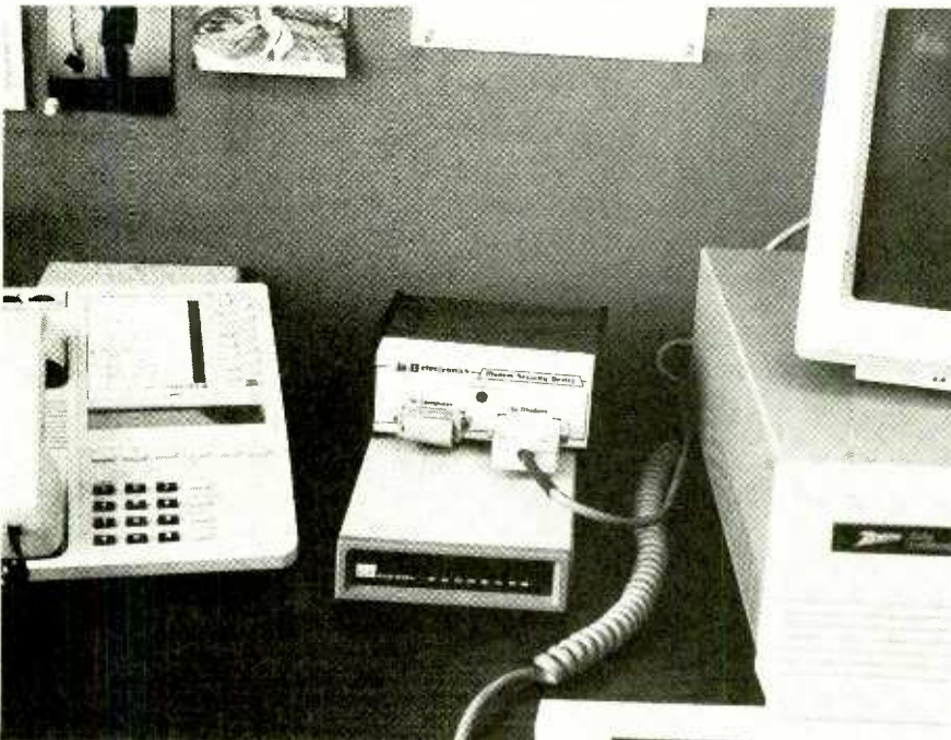
The MSD is shown sitting on top of an ADC MDI202 modem. Its small footprint takes minimal space. The MSD can be situated out of sight since, once installed, it needs no human direct control. Its front-panel LED is useful only during installation and orientation.
