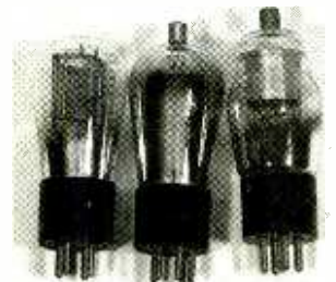
Fig. 6. By the early 1930's, four-, five-, six-, or seven-pin tubes like these (some having grid caps) began to appear.
