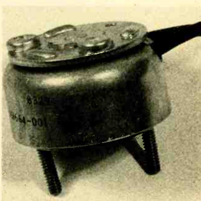
The Auto Feeder uses a rotary type solenoid (SOL1), which draws about 400 milliamperes when energized and is operated from the unregulated 12-volt supply, to eliminate any effects its current drain might have on the regulated 8-volt power supply. When this rotary solenoid is energized, the circular plate on top rotates about 20 degrees. On de-energizing, the circular plate returns to its original position.
