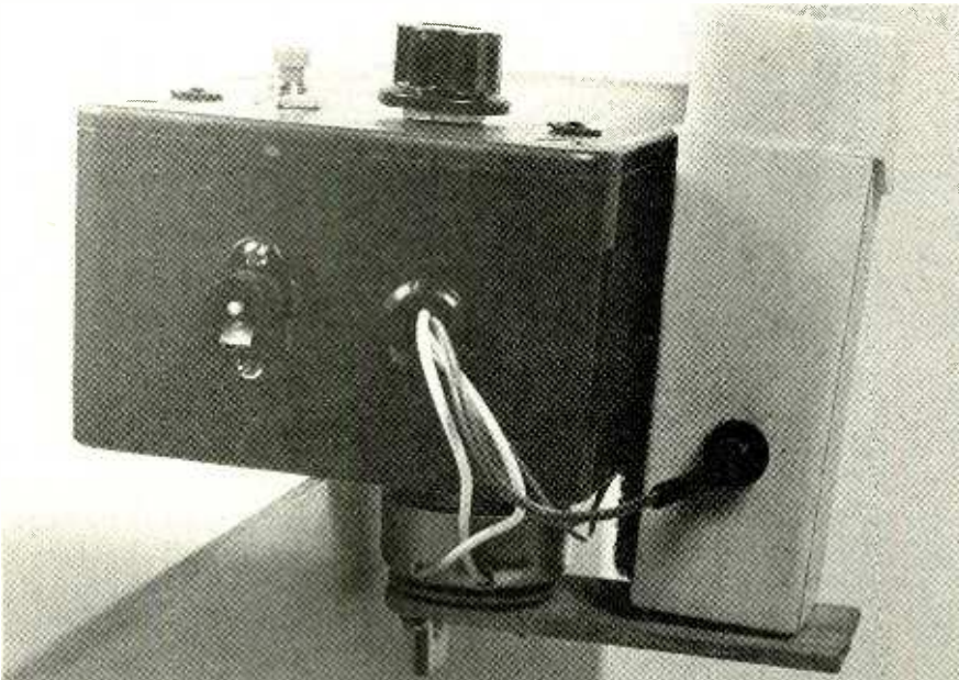
The solenoid mounts underneath the project enclosure. One end of a wooden flipper mounts on the solenoid's rotating circular plate, the other end rests under a fish-food bin, which has a hole in its bottom. When the solenoid is energized, the flipper moves away from the hole, and fish food falls through the hole into the fish tank. In addition to automatic feeding, you can manually feed your fish by pressing S1 (FEED).
