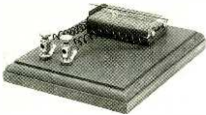
One very simple Hughes-type microphone can be made from two razor blades and a slim stick of graphite, or, in this case, an automatic-pencil refill. The system is mounted on a couple of wood blocks. Binding posts have been added to facilitate wiring.
