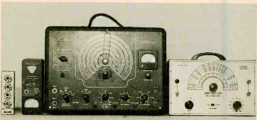
A typical grid-dip oscillator, RF sweep-generator, and audio oscillator. Units like these can be found at most hamfests for around $10.
