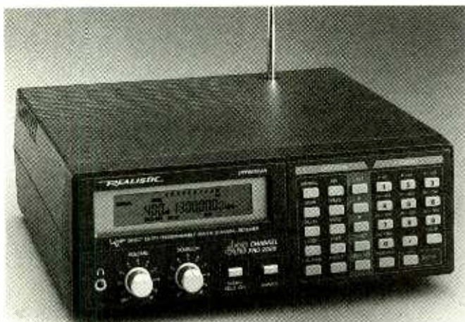
A worthy successor to the Realistic PRO-2004 and PRO-2005 , the new PRO-2006 adds “Hyperscan,” which allows you to search and scan at two impressive speeds: 26 and 13 cps.
