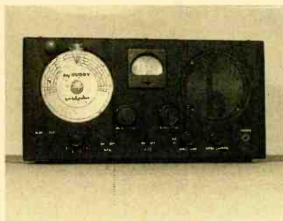
The Hallcrafters S-19R Sky Buddy was a budget six-tube receiver introduced in 1939. It will still do good work on the lower bands if backed with a good audio filter.
