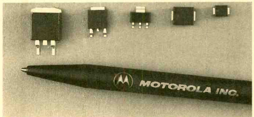
These case styles are used for power applications (power-transistors, regulators, high-amperage diodes, and such).
