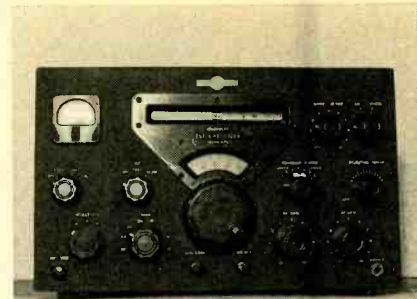
Few people would argue that the Collins 75A-4 isn't one of the best receivers ever made. It had Collins mechanical filters, the Collins super-stable tuning system, a bunch of other features and a price tag of $695.
