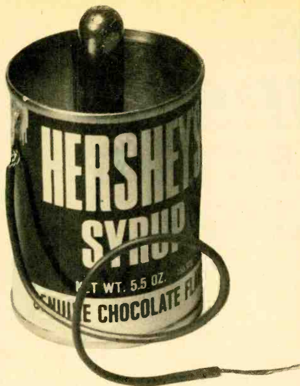
This metal can is filled with a sodium chloride solution. The can is then positioned so that the "rotor" can freely turn within it.
