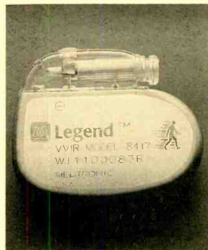
This is a small, light, implantable pacemaker designed to adapt its rate of impulses to the needs of the wearer. It can record information about the heart and "talk" to a physician about it when requested. The physician can then fine-tune the pacemaker for the user.
