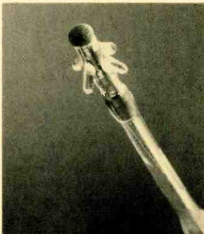
To reduce the battery drain in implantable pacemakers, a new steroid-eluting lead reduces pacing thresholds by reducing myocardial inflammation.
