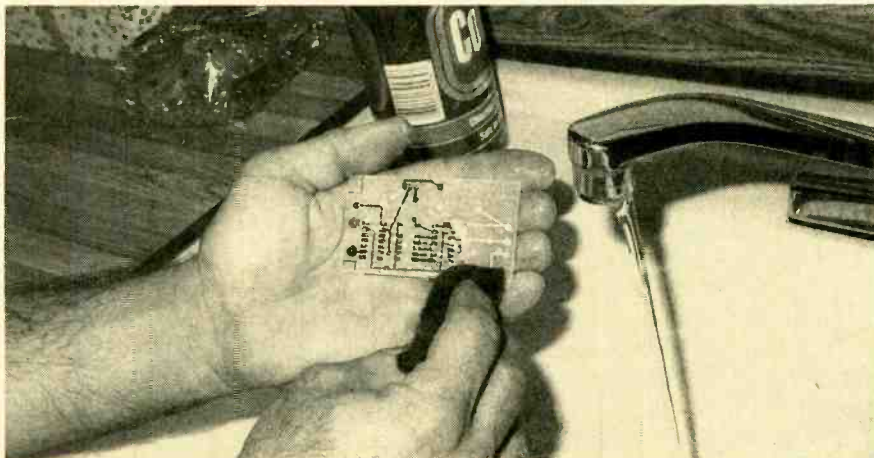
After checking to see that all excess copper has been completely removed from the blank, remove the toner resist from the copper traces using a plastic scouring pad and household cleanser. If you don't mind the added expense, there are solvents that can be used for that purpose.
