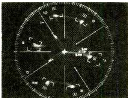
While color accuracy was just about perfect, the colors in the yellow, green and cyan areas were very slightly undersaturated as indicated by the fact that the light spots for those colors are somewhat inboard of the target cross marks.
