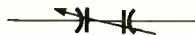
Fig. 9. This is the schematic symbol for split-stator capacitors. They often find application in antenna tuners.
