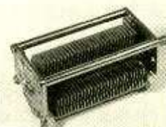
This is a simple single-section air variable capacitor. They can find use in any circuit that requires capacitive tuning at reasonable voltages.
