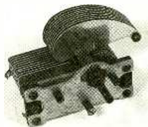
An offset shaft and unusual rotor plates allow this capacitor to track frequency (or wavelength) in LC-tuned resonant circuits.
