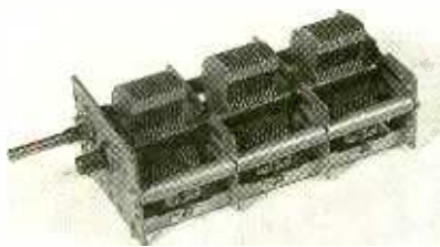
A multi-section variable capacitor is basically several capacitors mechanically ganged to the same shaft. Thus, they move in unison.
