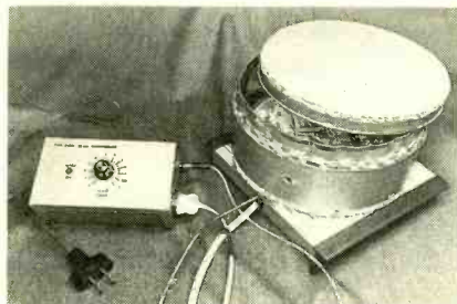
Here's one of the author's applications for the controller—a home-made oven used to dry PC-boards in less than one-half hour.
