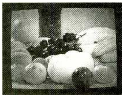
Fig. 1. At a signal strength of 1000 \mu V, the receiver displayed a top-quality picture
