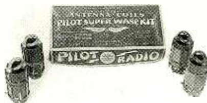
Here are two of the Wasp's five coil sets. The original box for the antenna (RF amplifier) coils is in the background.
