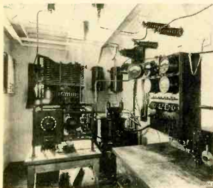
This Navy 5-kW shipboard arc transmitter/receiver station operated on a frequency from 100 to 250 kHz.
