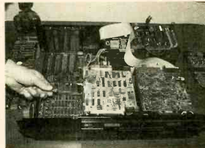
To remove the diskette drive, unscrew the two mounting fasteners, either on the left side of drive A or on the right side of drive B. To remove the drive A screws, you will have to remove the nearby adapter cards first.
