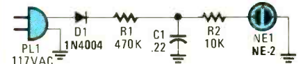
Fig. 6. The Wall Finder is nothing more than a flashing line-fed neon lamp.
