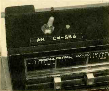
Once switch S1 is in place, it's a good idea to label the switch positions on the outside of the receiver's enclosure. Removing power from the circuit, by flipping S1 to the AM position, effectively disconnects the Adapter from the receiver's detector diode.
