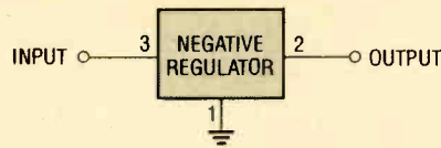
Fig. 4. This is the negative-voltage regulator symbol (note that the pin-outs are different with respect to positive regulators).
