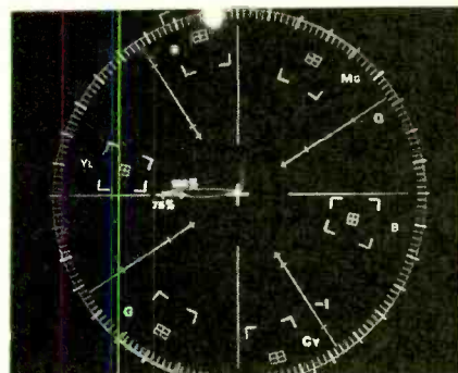
This vectorscope photo was taken when the camcorder was recording a red field. The white "spot" seen at the top of the photo represents the phase angle and the degree of saturation of the red color. Ideally, that spot should fall exactly in the center of the cross-mark labeled "R" (for Red).
