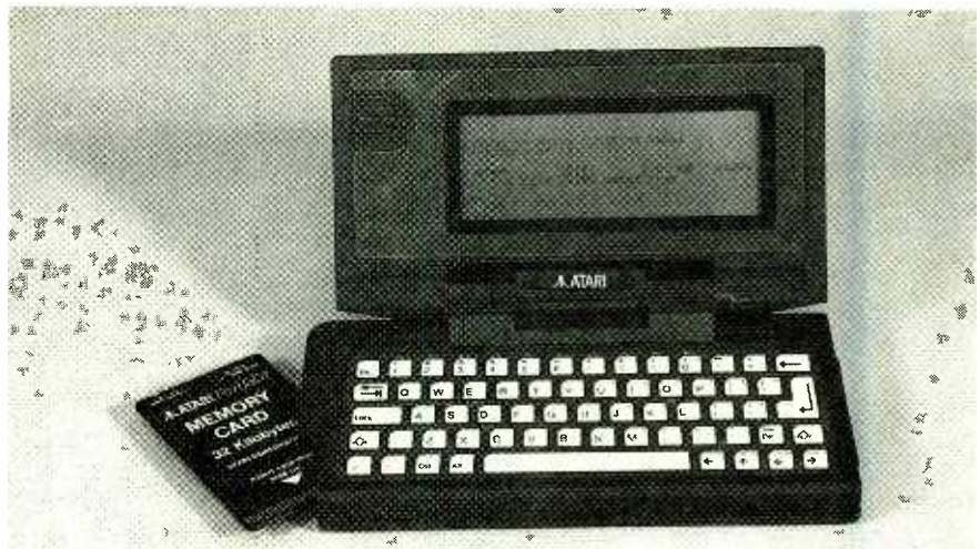
Sophisticated micro-miniaturization technology was used to make the Atari a one-pound unit, which is slightly smaller than a video-tape cassette. The thin memory card snaps into a side port. Note the piano-key-like contacts at the bottom of the card.
