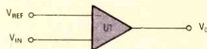
Fig 1. A basic op-amp comparator is shown here. Because the op-amp is operated in an open loop configuration, the input voltage difference required to toggle the output from one state to another is very small.
