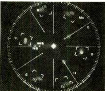
In the case of the PAL tests, the vectorscope indicated a double set of vectors; one correct, one somewhat displaced. Since the effect was not viewed when observing the actual color bars on the monitor, APEL believes the odd display was caused by the difference between U.S. AC frequency and the PAL line-repetition rate.
