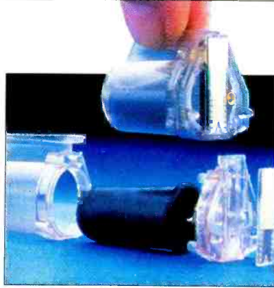
The unique print-head/ink-bladder design of HP's Thinkjet.
