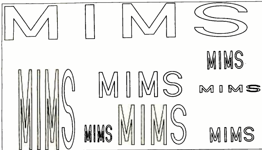
Fig. 7. Changing the plotter's scale under program or front panel control alters the dimensions of the letters drawn by the program in Listing 2.
