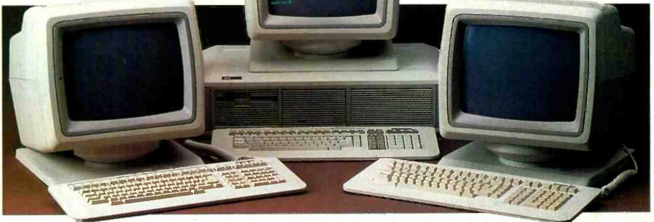
A LAN can join 63 of the pictured MAI 2000 desktop units, each of which can handle 14 users.
