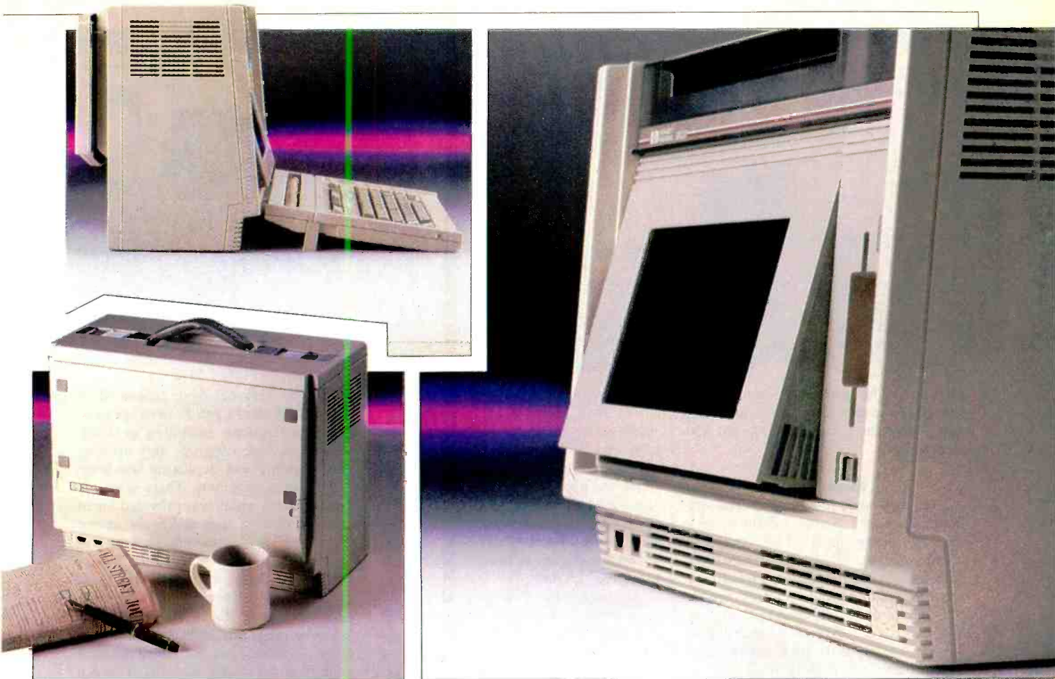
Above, left: HP-IPC in profile. Detachable keyboard is clamped to front of case (below, left) to protect unit while in transit. Right: Flat panel display pops out at a convenient viewing angle at the touch of a lever. Disk drive is at right of display.
