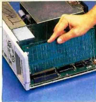
The 1000 can accommodate three IBM-compatible expansion boards.
