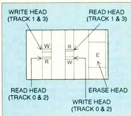
**Fig. 3. Read-after-write head.**
