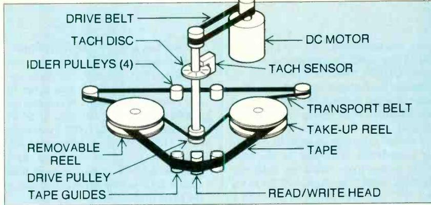
**Fig. 6. Interdyne's device uses a self-threading system.**
