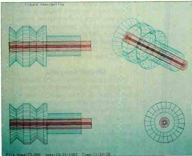
In the three photos at the left, the Space Tablet is used to draw a pulley. Thirteen digitized positions are required—one to identify the axis and 12 for the ring structures with the same axis. In the center photo, the dimensions and text labels are added to the drawing. At the immediate left is the plotter output showing top, front, and isometric views of the pulley.
