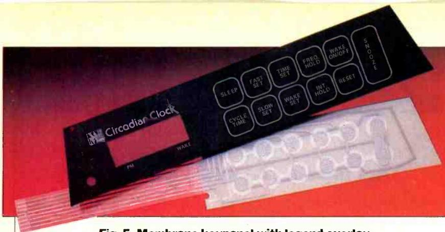
**Fig. 5. Membrane keypad with legend overlay.**
