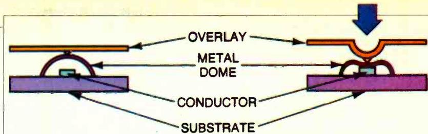
**Fig. 4. Metal dome in keypanel gives tactile feedback.**
