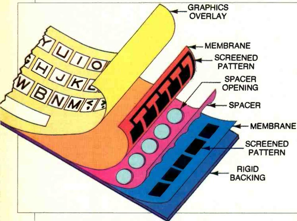
**Fig. 6. Patterns screened on membranes form switch contacts.**
