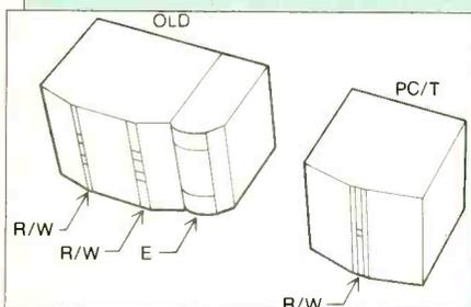
found in the form of the QIC standard. The standard calls for a head with two read gaps, two write gaps and an erase gap—five gaps total. As a result, the head is costly, and maintaining azimuth between the gaps proves difficult. Thus you'll find a simpler head, with a single gap, in Tallgrass's own tape drives. The head actually overwrites a tape, rather than erasing it.
