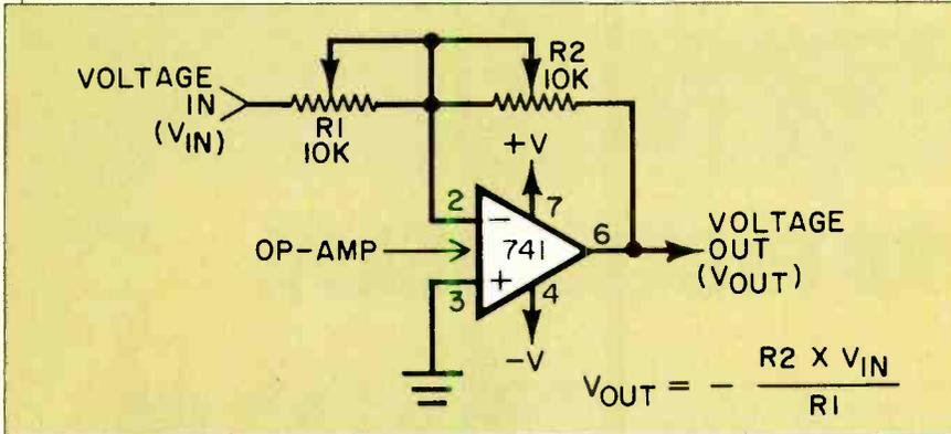
**Fig. 4. Basic operational amplifier variable resistor multiplier.**
