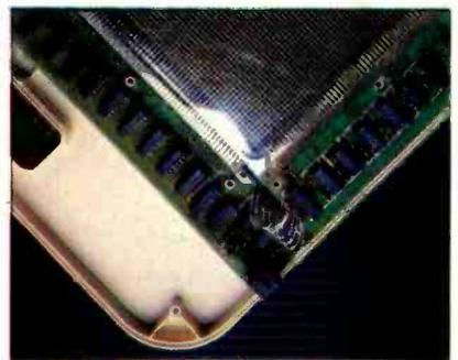
The powerPad uses two plastic grid sheets to form 100 switches per square inch or 14,400 switches per pad.
