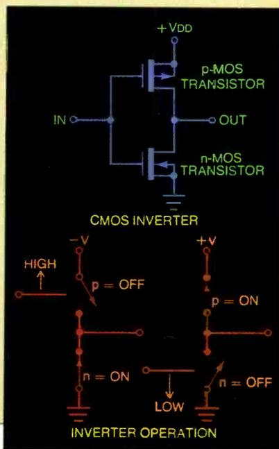
When low operating power is combined with high-density, multi-purpose CMOS ICs, the savings come in the form of less costly support components and raw materials consumption, which results in minimized "real estate" required for the circuitry.
