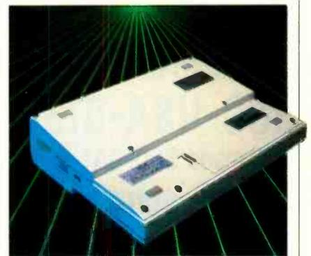
**RAM disk attached to the PX-8.**
