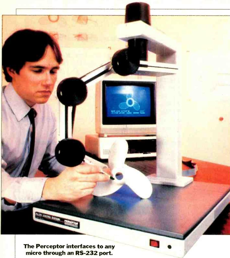
**The Perceptor interfaces to any micro through an RS-232 port.**
