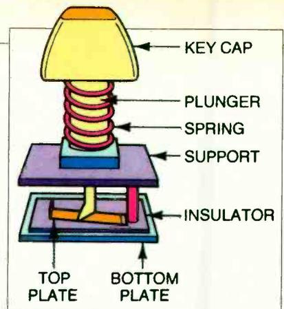
**Fig. 1. Capacitance keyswitch.**
