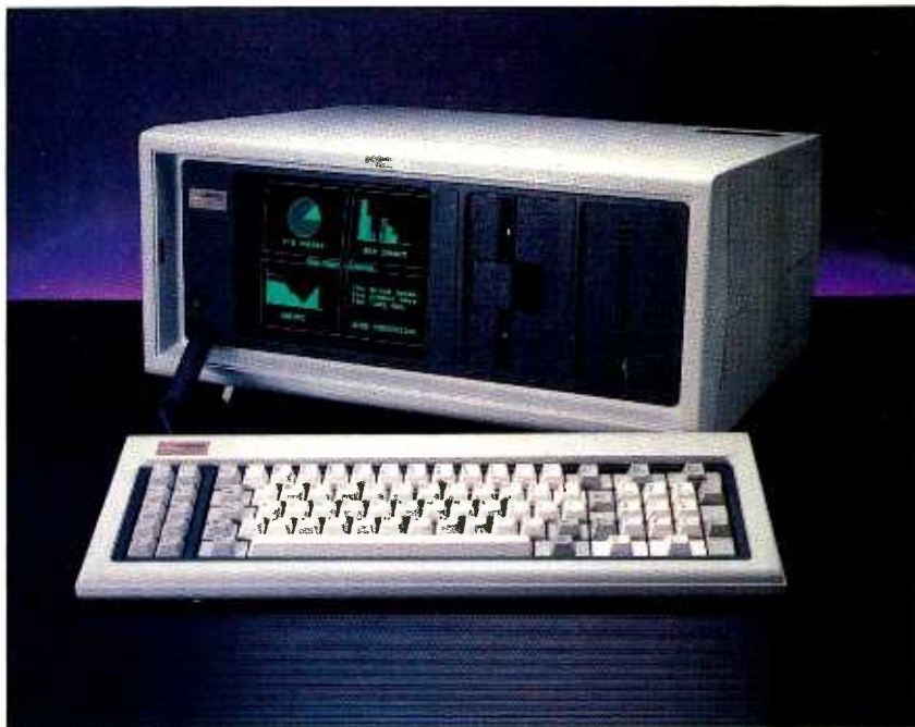
The Compaq Plus includes a 10M-byte hard disk and 9" monitor.
