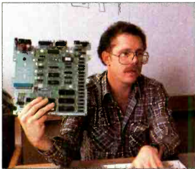
Engineering chief Peter Quinn holds Apple IIc's only board (above). Robert Gemmill describes vent slots (right). Far right are ports on back and mouse.
