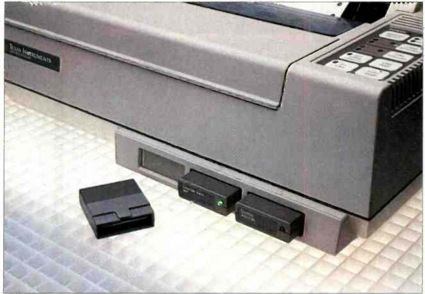
Front-panel slots accept up to three ROM modules for selecting a variety of character fonts for printed text.
