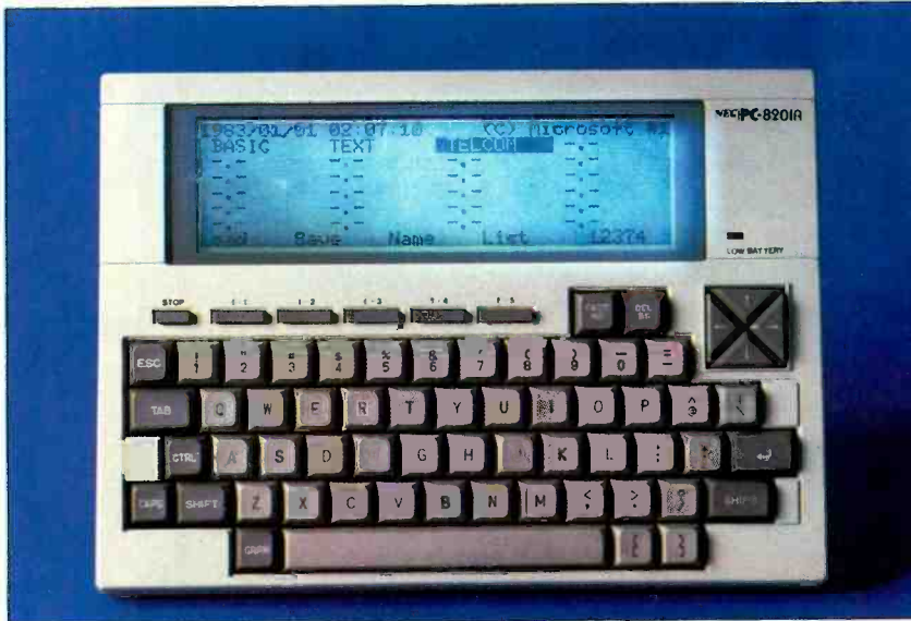
The NEC has a 40-character by 16-line LCD screen.
