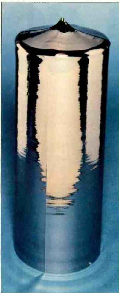
A 6" pure silicon ingot, before being cut into wafers for fabrication.
