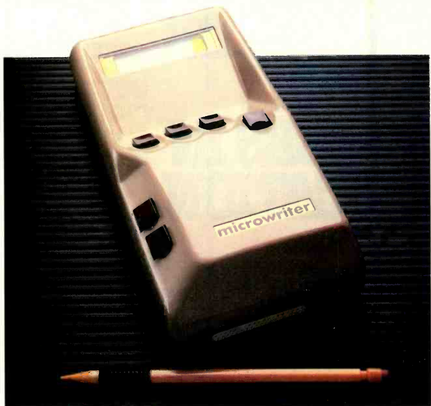
Microwriter has a unique six-key entry system.
