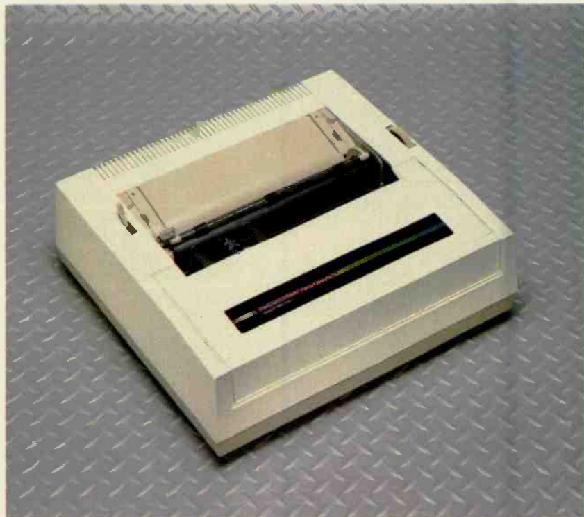
The daisy-wheel printer houses the system power supply.
