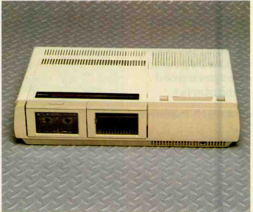
Memory console with data drives and game cartridge socket.
