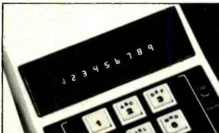
LED Display Shows No. Being Dialed.
