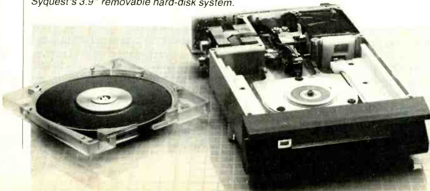
Syquest's 3.9" removable hard-disk system.
