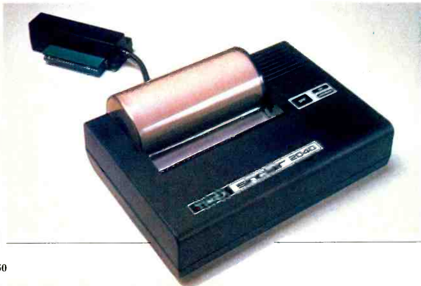
Timex Sinclair 2040 printer works with either TS1000 or TS2000.
